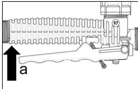
Releasing the shut-off valve stops the spray process.
